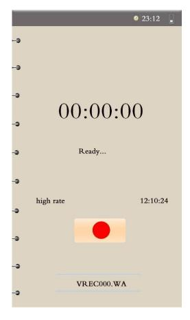
**Start/Pause Recording –** Choose "Record" from the Main Menu to enter this interface. When in the Recording interface, press "**M**" to start recording, pause recording, or to switch recording quality.
